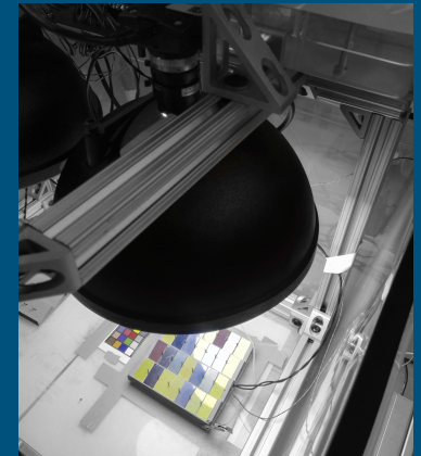
Age Testing w/image capture (5 days, 85°C, 85%, 0.15Sun)
